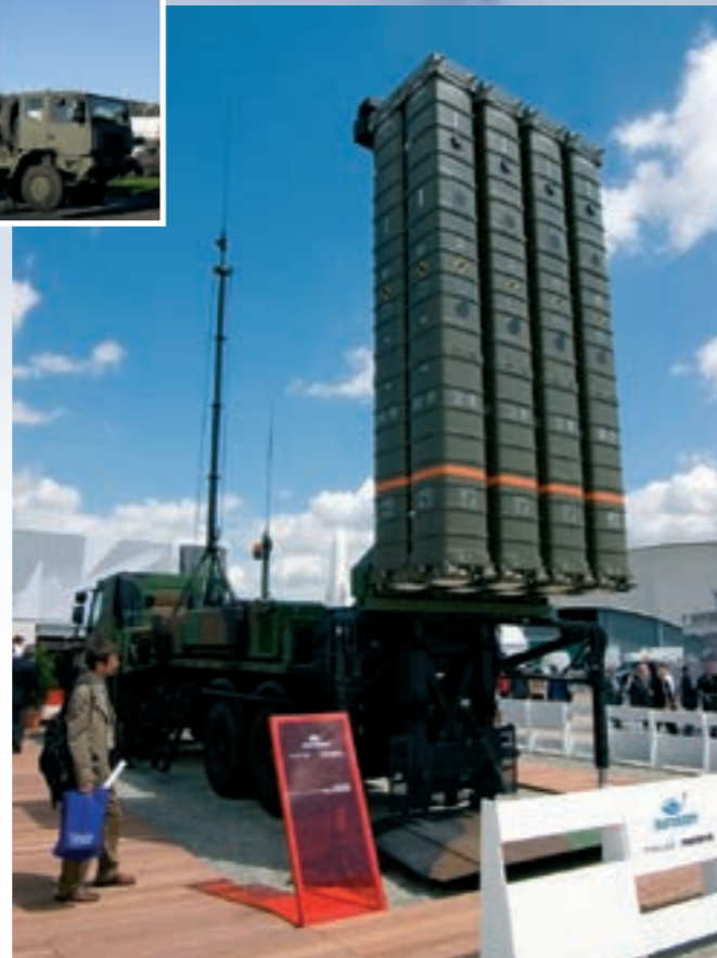
■ During transport, the launch tubes are horizontal, but once in positions, they are erected for the vertical launch.
